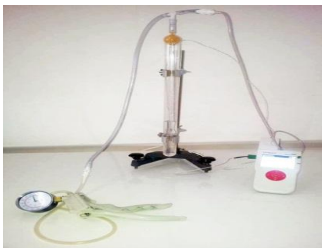
2-rasm. Simob tomchilarini yig'ish va dastlabki gaz hajmi ( V_0 ) ni o'rnatish.
